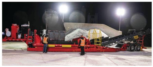
Equipped for an hourly transfer rate upward of 200 yd., the TranzLoader is sized to meet concrete plant output and contractor placement requirements on remote or specialized sites not warranting portable plant ramp up. Ozinga Bros. has proved the economy and efficiency of deploying dump trucks from batch plant to TranzLoader tub, then enlisting mixer trucks for final concrete placement.
