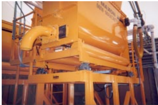
Above: On a similar project for the Oak Ridge Uranium Complex, Maxon provided two Mini-Maxcretes mounted on elevated platforms for discharge into specially designed containers. The Mini-Maxcretes were equipped with load cells between the mixer frame and the platform to monitor product weight. In addition, the standard discharge gate was replaced with a guillotine valve and 90 degree elbow for discharging liquids.
