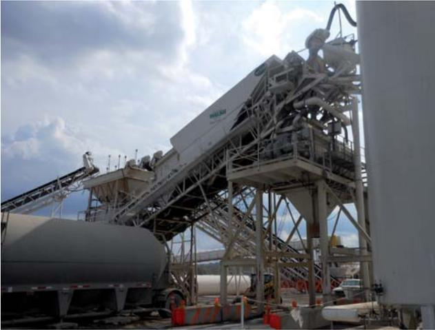
Central mix batch plant with twin shaft mixer was erected approximately 1,200 feet from the powerhouse concrete placement.
