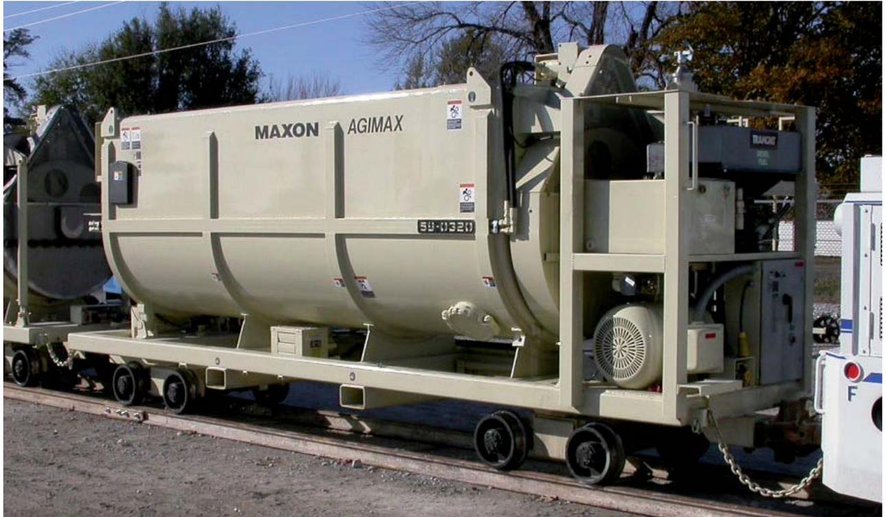
The **Maxon Agimax** is designed to transport, agitate and place concrete in low profile underground applications, where discharge heights will not allow a full hoisting body similar to the **Maxon Agitor**. When working in small-bore tunnels, the Agimax offers many advantages not available with conventional agitator cars.
