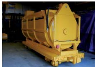
Additional features for the Agimax include two (2) hoist cylinders to lift the body during discharge. The Agimax shell is constructed of 1/4" AR300 abrasive resistant steel for maximum wear.
