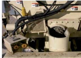
The Agimax discharges through an 8" diameter hydraulically operated knife valve. The valve is adjustable for wear to reduce leakage, and can be feathered or fully opened for discharge speeds from a trickle to 6 cubic yards per minute.
