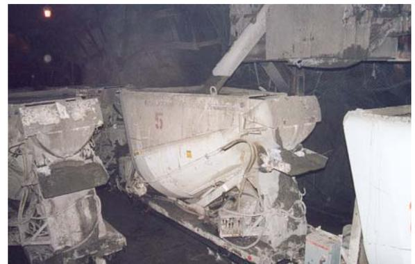
*Open top Agitor accepts concrete from drop pipe*
