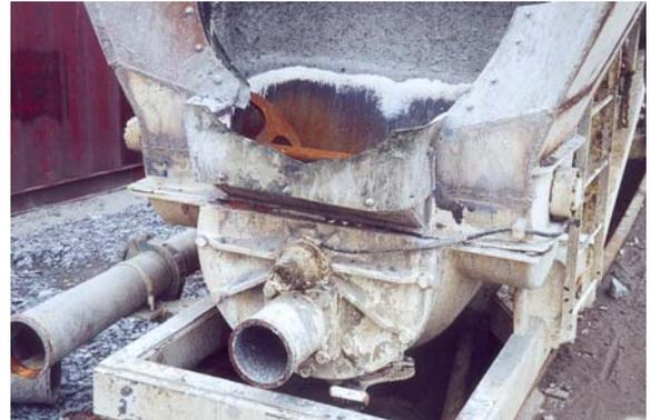
*Concrete pump (shown above ground) with Modified hopper for exact fit to Maxcrete*
