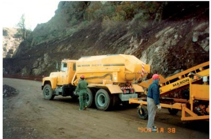
*Truck-mounted Maxcrete transporter feeds concrete to....*
