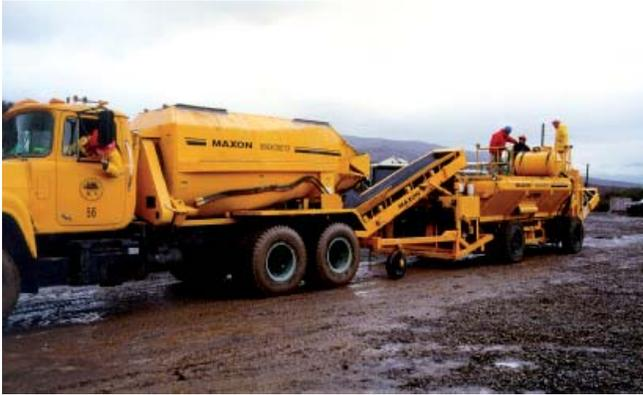
*The Mobile Maxcrete (right) accepts a load on its charge belt while pushing the Truck-Mounted Maxcrete.*
