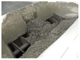
View inside Surgecrete: Bi-directional auger moves even the stiffest of concrete mixes to the hydraulically operated discharge gate, and onto the 36" discharge belt.
