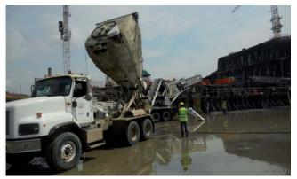
Maxon custom insulated the Agitor bodies to transport the super cooled concrete (ambient temperatures can exceed  $90^{\circ} \text{ F} / 30^{\circ} \text{ C}$ ).
