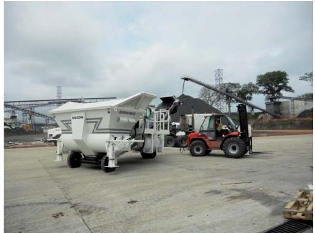
Versatile Maxon Surgecrete with tri-axle trailer configuration allows for easy towing to different placement sites on the project. Once in position outriggers provide for quick setup.
