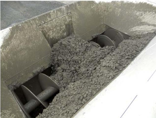
View inside Surgecrete: Bi-directional auger moves even the stiffest of concrete mixes to the hydraulically operated discharge gate, and onto the 36" discharge belt.
