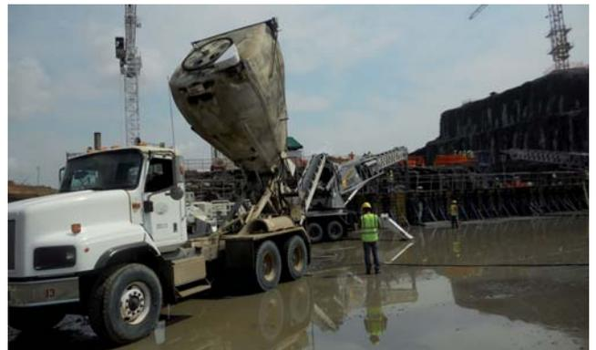
Maxon custom insulated the Agitor bodies to transport the super cooled concrete (ambient temperatures can exceed 90° F / 30° C).
