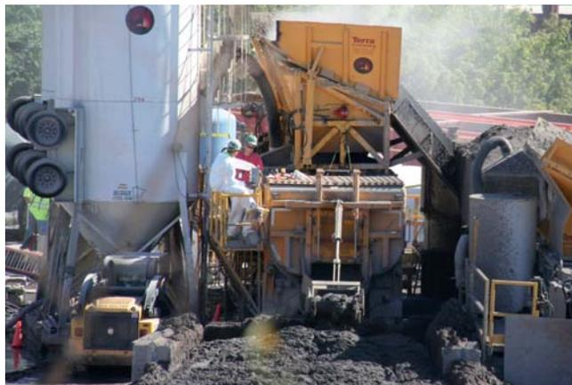
*16 cubic yard twin shaft Maxcrete (shown with grizzly mounted above) continuously mixes sediments with portland cement and discharges solidified end product.*
