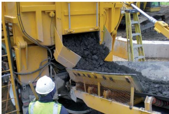
*Large hydraulic gates on both Maxcretes allow for rapid discharge of the end product. Maxon supplied each Maxcrete with a 20' Maxon belt conveyor with hydraulic lift to allow easy stockpiling of solidified product.*
