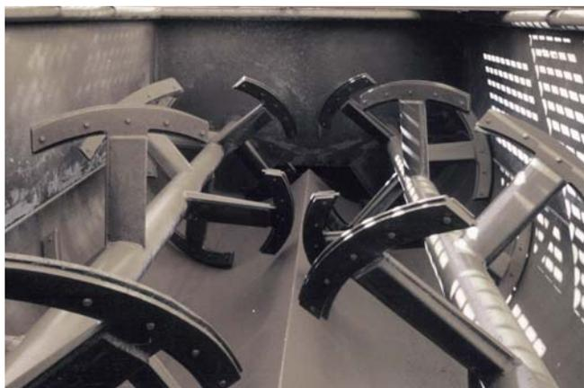
*Twin agitation shafts inside 16 yard Maxcrete allow continuous processing. The counter rotating shafts increase retention time in the mixer, allowing the Maxcrete to be simultaneously loaded with sediment/cement while discharging a homogenous solidified product.*
