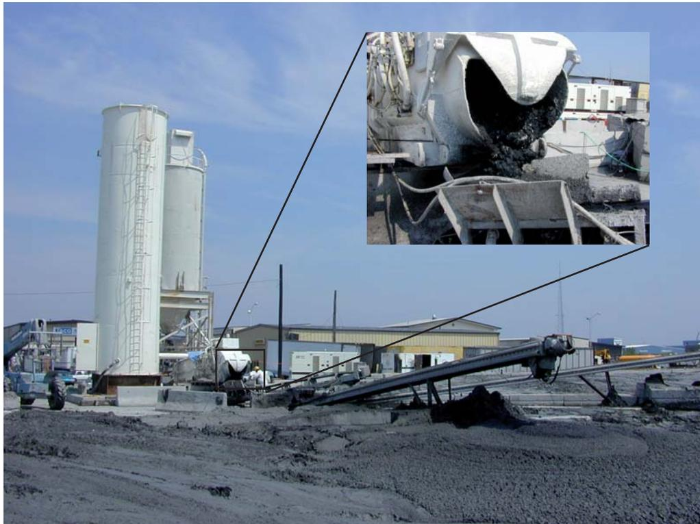
10 cubic yard Maxon Maxcrete is charged with dredged soils from the pump barge while continuously blending with dry reagents. Maxon equipped the Maxcrete with a 20' discharge conveyor and three 50' placing conveyors, allowing the system to distribute the flowable mixed material onto one of three concrete pads. After drying for three days, the solidified material was spread over the vacant lot creating a cap on the former brownfield site.
