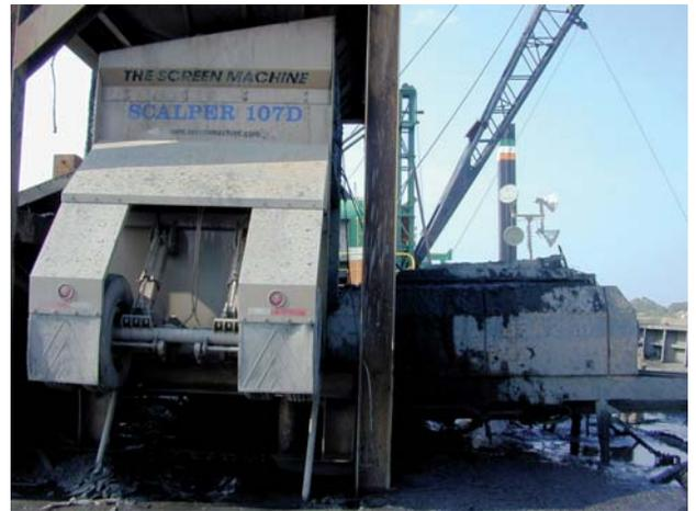
Dredged material is placed into an elevated heavy-duty screen plant which directly fed a trailer mounted concrete pump on the barge.
