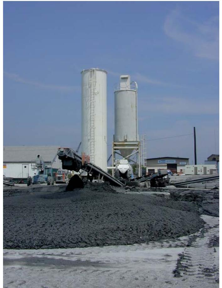
Production rates approached 100 cubic yards hour, with the limiting factor being the ability to have the dredge/pump barge keep up with the pace of the Maxcrete solidification system. "The system supplied by Maxon worked great," commented Tom Trafton of Dry Dredge. "The Maxcrete allowed us to modify our mixing design and retention time in the mixer based on moisture content, so we could ensure the material would achieve the consistency we needed by the third day."
