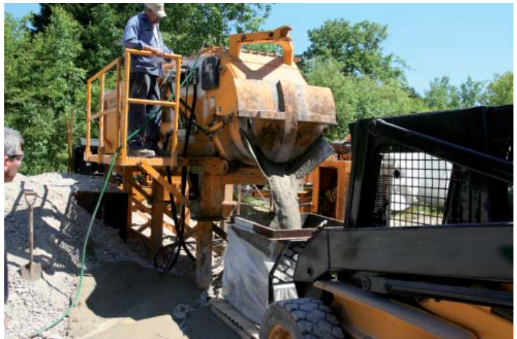
MAXPRO SPU 7.0 Pharmaceutical Waste Processing System. Unit shown discharging processed waste into a plastic lined form box, handled by a fork lift truck. Once the encapsulated pharmaceutical waste solidifies (approximately 4 hours) the form box is stripped and reused, and the block of encapsulated pharma waste is hauled to the local landfill.
