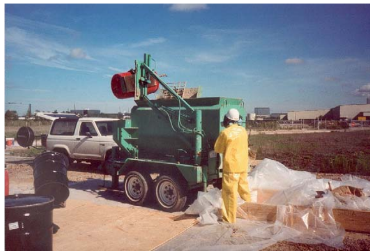
MAXPRO SPU 2.0 Pharmaceutical Waste processing system. Portable unit, trailer mounted for easy towing behind one ton pickup truck. MAXPRO includes hydraulic barrel loader, that will grab, lift, swing and rotate drums up to 55 gallon or 800 lbs capacity.
