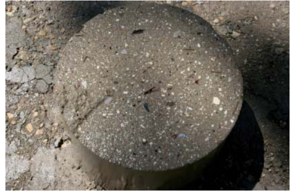
A cross section of a test cylinder is shown with pharmaceutical waste 24 hours after processing.
