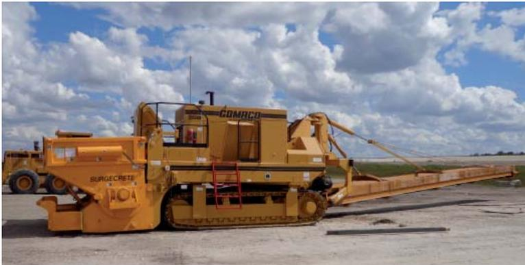
To place soil cement for the lower steps of the walls, Kiewit used two modified Gomaco 9500 placers. The existing hopper on the 9500's included a 12" screw designed to handle concrete. In initial trials with the 9500 placers the soil cement material would bridge in the hopper, slowing production.
